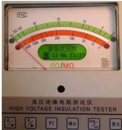
Can save the current date (year, month and day) and time ( left and right key adjustment),press "confirm" button to save and return to the main menu.
