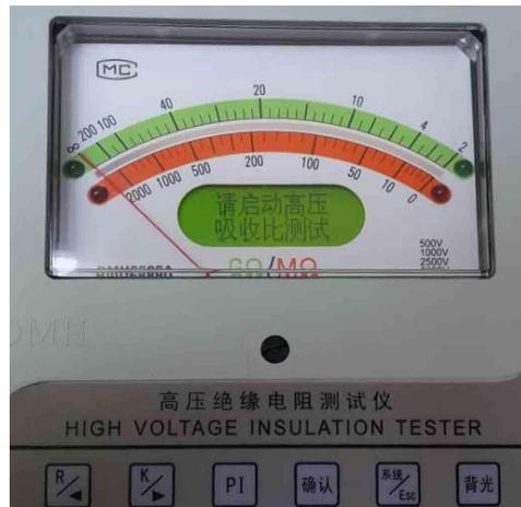
Start high pressure tested, the following diagram has been testing 20S, The test voltage is 1.00kV, test resistance is 1.02 GΩ, 15 seconds values have been locked in 1.02 GΩ.
