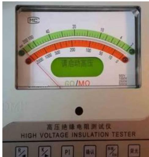
According to the menu prompt start high voltage button (13) output high voltage test.
