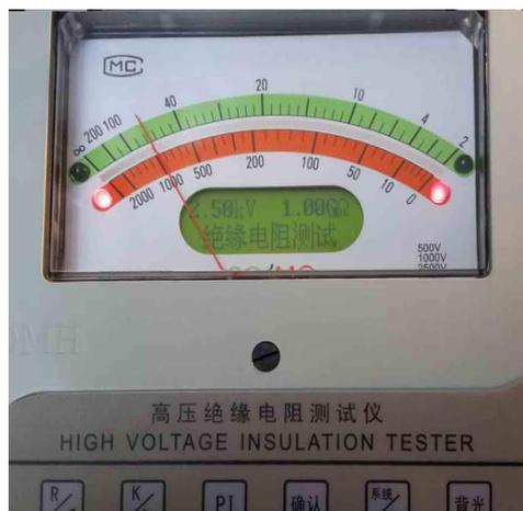
Now close the high-pressure output, menu prompt whether to save the current test data. As shown in Fig:
