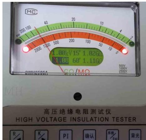
Tested voltage 1.00KV, 15 seconds to test resistance value is 1.02 GΩ, 60 seconds to test resistance value is 1.11 GΩ, absorption ratio test results is 1.08. If you press "ESC" key to exit, can automatically save the current test results and the test time, and return to the main menu.
