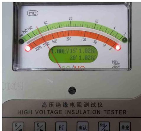
Absorption ratio test time after 60 seconds, as below shows, Closing high voltage output
