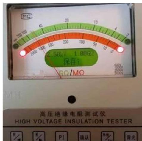
Press "confirm" button to save the current Conventional insulation resistance testing results.
