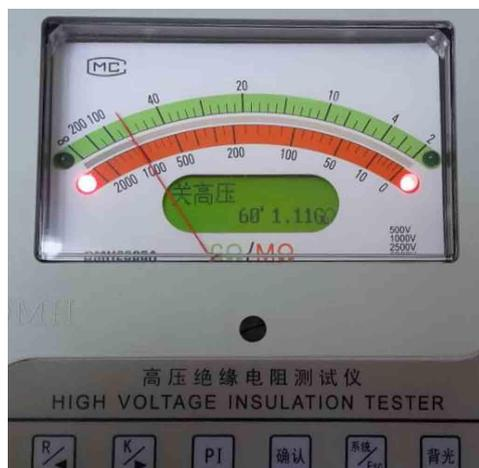
Close the high-pressure output complete absorption ratio test, test results show as below
