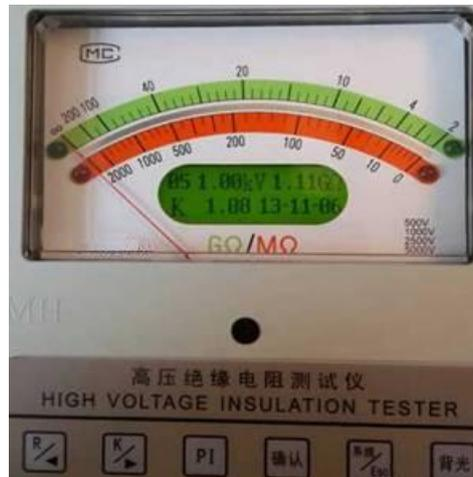
Can view the data of storage, this time press left key or right key can turn to front or next record.
