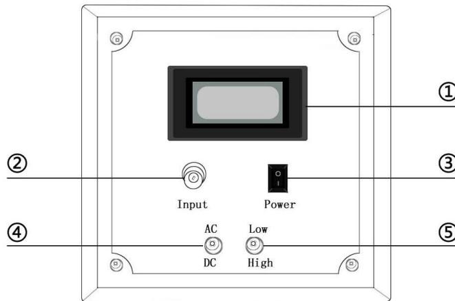
**Figure 3 Low voltage display meter**
